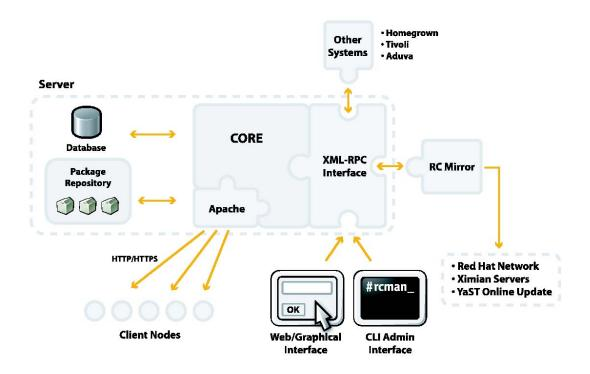
Similarly, the client daemon, rcd, uses an XML-RPC interface to accept commands from rug and red-carpet, remotely or locally. Additional modules provide the client with the ability to interact with the ZENworks Linux Management server for extended functionality.
