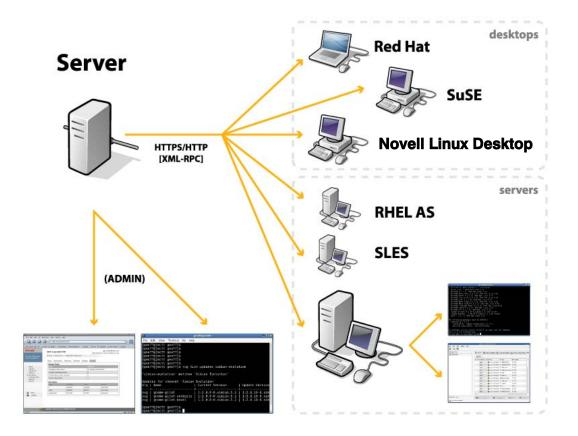
The ZENworks Linux Management server uses an XML-RPC interface to communicate with a variety of clients and other systems. Although remote access to the XML-RPC interface is possible, the ZENworks Linux Management server components are intended to run locally on the ZENworks Linux Management server, and are supported only when running locally.
